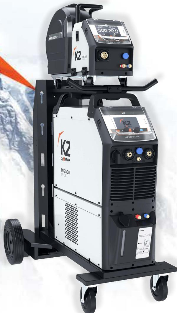
**K2 MIG 500 DPULSE** is an inverter-based three-phase (IGBT) multi-process welding machine for MIG/MAG with Pulse and Double Pulse, (Lift) TIG, and MMA applications. Experience precise control, sophisticated user functions, accurate welding settings, and real-time monitoring through a clear LCD display.
