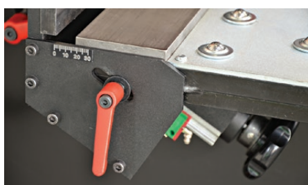
Simple setting of bevel width
