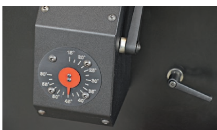
Precise bevel angle adjustment
