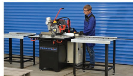
Auxiliary tables to accommodate long workpieces
