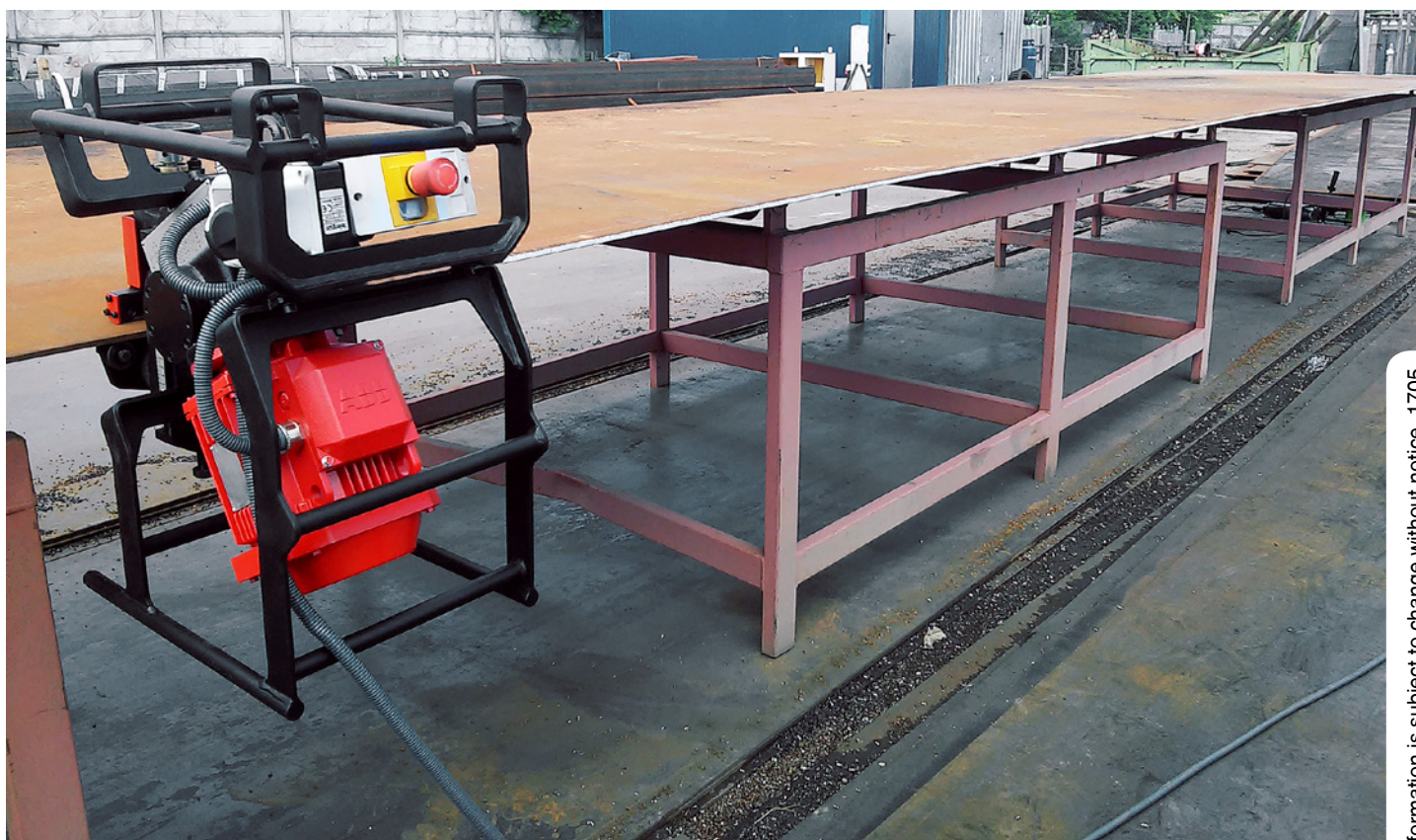
ABM-14 runs along a plate automatically
