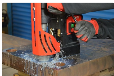
Milling capacity up to 70mm (2-3/4")
