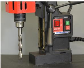
Adapter 3/4" x 1/2" 20 UNF, Drilling chuck 1/2" 20 UNF
