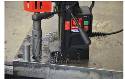
Milling capacity up to 55 mm (2.17")
