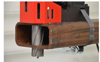
Starting point of milling up to 50 mm (2")
