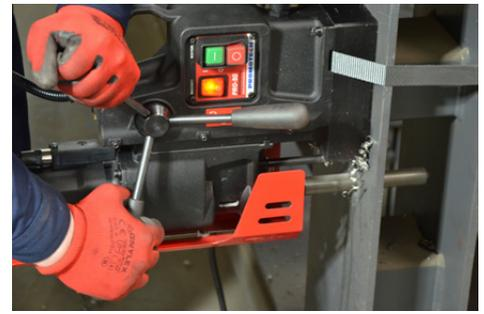
Drilling capacity up to 23 mm (0.91")
