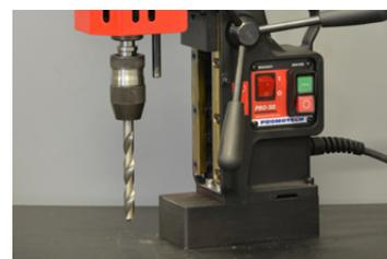
Adapter MT2 x 1/2" 20 UNF, Quick change drilling chuck 1/2" 20 UNF
