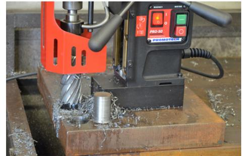
Milling capacity up to 50 mm (2")
