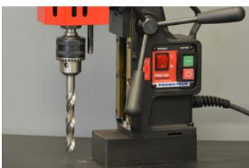
Adapter MT2 x 1/2" 20 UNF, Drilling chuck 1/2" 20 UNF
